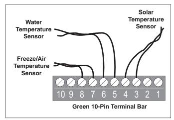
Figure 17. Temperature Sensor Wiring for a Pool/ Spa Combination
